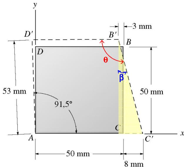
$$(\gamma_A)_{xy} = 90^\circ - 91,5^\circ = -1,5^\circ = -1,5^\circ \times \frac{\pi}{180} = -0,026179939 \text{ rad}$$
